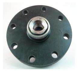
The Poly-Cam Female Header Fitting (Series 799) is a barbed mechanical design fitting which is hydraulically compressed into the polyethylene or pipe quality copolymer material. The fitting is fused onto the HDPE blind flange and includes a compression ring for reinforcement.
