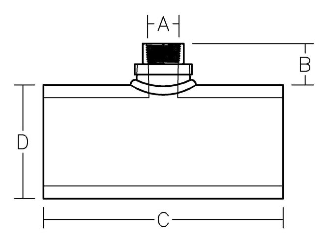
Fully pressure rated • Standard SDR sizes 7,9,11,17 Manufactured to ASTM D3035, D1599, D1598, D3350
